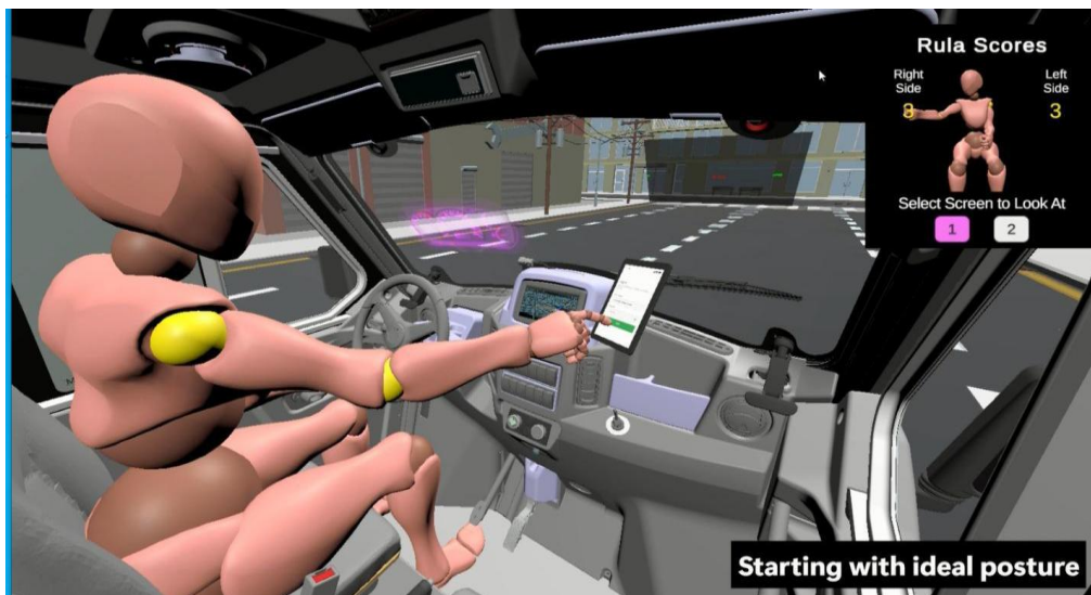
Figure 31: INTERACTION OF USER WITH HMIS AND THE XR PROJECTED INFORMATION ON THE WINDSHIELD THROUGH THE XRIVE TOOL
