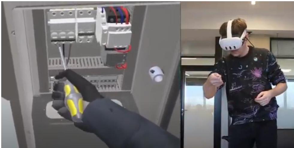
Figure 2. Manipulating a virtual screwdriver with MetaQuest 3 Hand tracking
